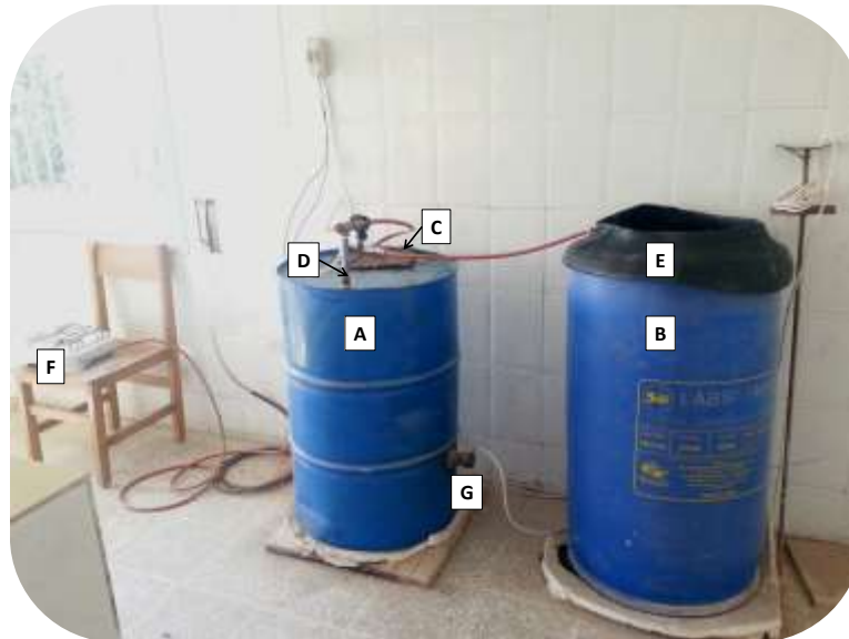
Figure (2): Laboratory designed digester used in this study. (A) Barrel to be filled with OMW mixture, (B) Barrel for OMW storing, (C) an opening for filling the barrel with OMW, (D) a gas outlet, (E) a tire to contain the resulting biogas, (F) a household stove to test biogas combustion, (G) a water heater.
