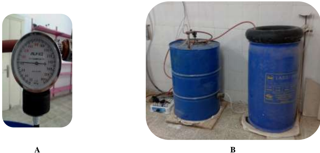
Figure (4): the laboratory designed digester in the day 47 of the anaerobic treatment experiment. A: Pressure gauge showing an increase in biogas pressure, B: The biogas tire filled.
