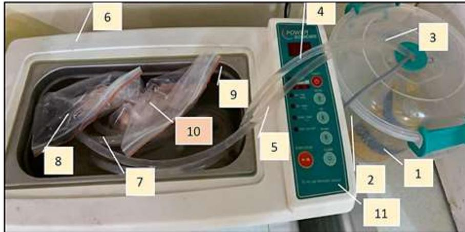
**Figure 1. pelvic ultrasound device provided with a heat exchanger.**
