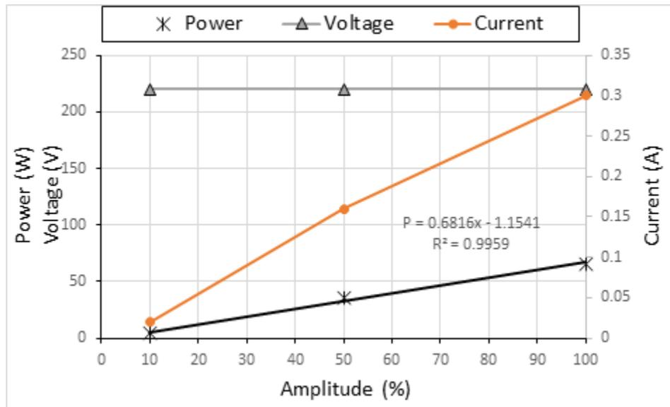
**Figure 2. The relationship between power (W), voltage difference, current, and percentage of power (%). Color Measurement:**
