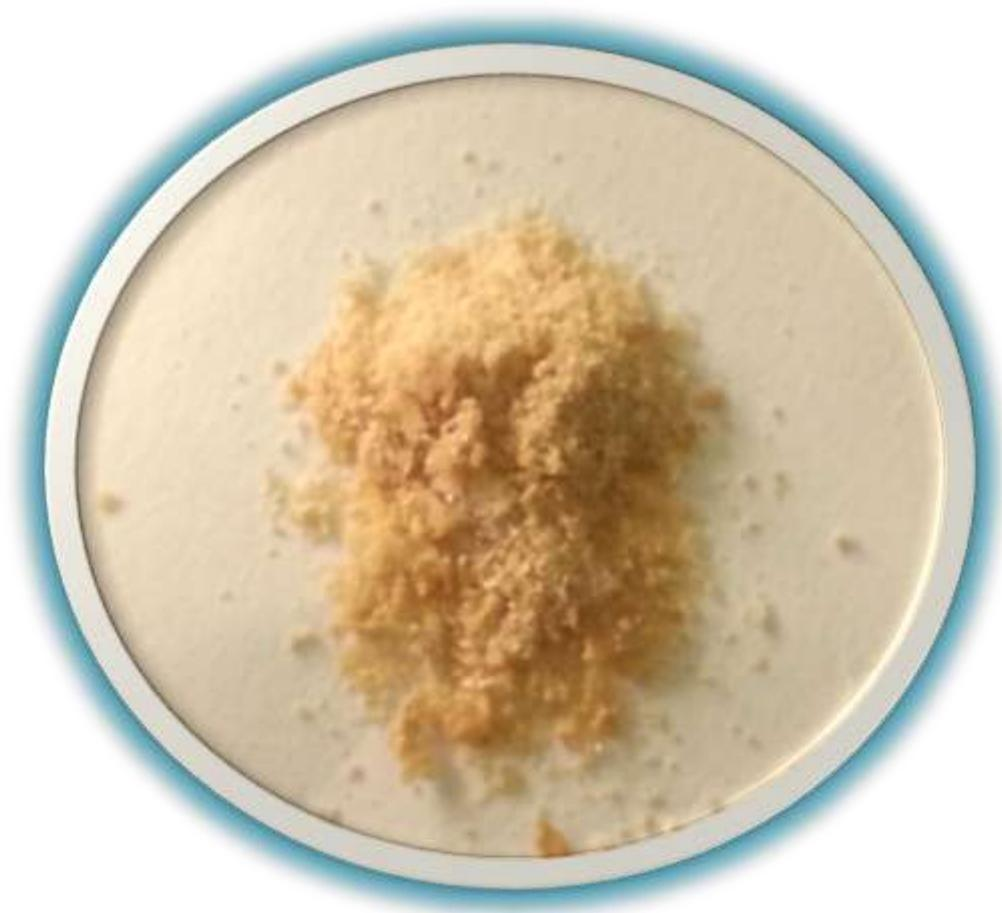
Figure 3. Extracted PHB crystals from *P. aeruginosa* DW7 by Sodium hypochlorite-Chloroform method
