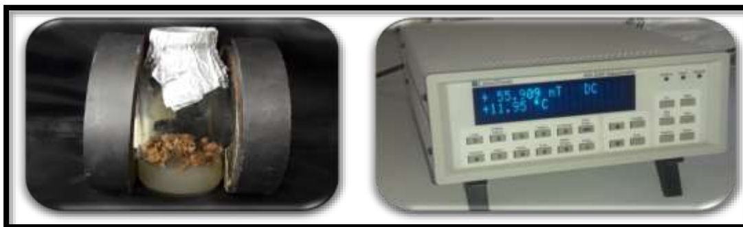
Figure(1): Magnetic field device used for exposure Explant and Callus cultures
